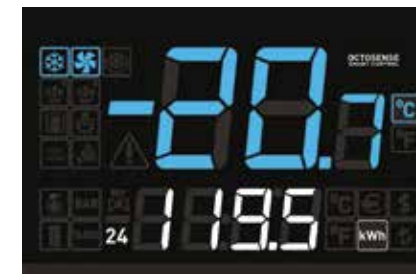
daily energy consumption (kWh)
