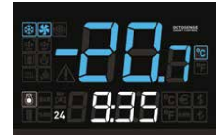
daily compressor operation time
