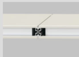
Wall joint 4 mm silicone gap
